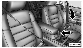
Inserting Latch Plate into Buckle
